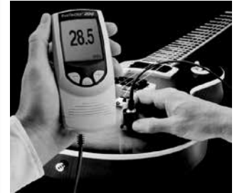
Measure paint, varnish, lacquer, etc. on wood products including cabinetry, furniture, flooring, windows and more.
