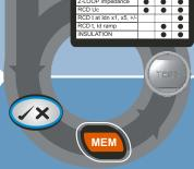
Save AUTO SEQUENCE® test results to memory, transfer results to a PC and create standardised test reports. The operator can save acquired test results to structured memory, under switchboard level or under circuit level, all at once. Run Eurolink PC program, transfer all acquired test results to a PC over USB or RS 232 connection, verify the data and print automatically generated test report.
