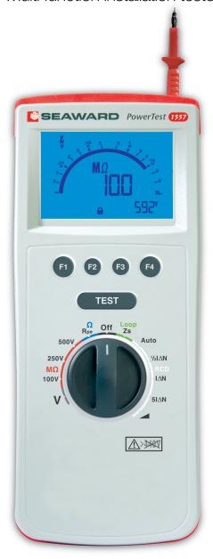
Thanks to a clever bit of design, we have included a cordless probe for use with the tester, meaning you can hold the tester and see the results at the same time. Weighing in at a mere 900 grams, it's light too. And it can do any test that you require at the turn of a knob, including Earth Continuity, Insulation (100v, 250v, 500v), Non-trip Loop Impedance, Line Impedance, RCD trip line, RCD trip current and voltage / frequency measurements.
