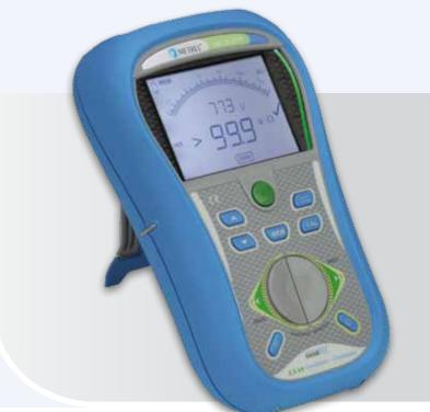
The MI 3121H Smartec 2,5 kV Insulation / Continuity is the portable measuring instrument for complete diagnostic testing of insulation and continuity measurements. Due to insulation resistance measurement with the test voltages up to 2.5 kV (measuring range is up to 100 G $\Omega$ ) and calculation of PI and DAR indexes the instrument is ideally suited for testing insulation of cable lines, current and voltage transformers, electric motors, etc.
