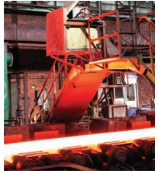
Steel Hot Strip Mill
